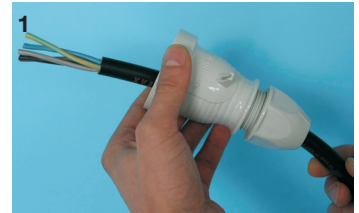
Remove approx. 35 - 40 mm of the sheathing from the cable (with 6 mm 2 45 mm) and feed it through the back part from behind. Cut off the non-conductive core.
